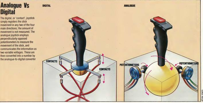
The digital, or 'contact', joystick simply registers the stick movement in any two of the four main directions: the amount of movement is not measured. The analogue joystick employs perpendicularly opposed potentiometers to measure the movement of the stick, and communicates the information as two variable voltages. These are then converted into a number by the analogue-to-digital converter
